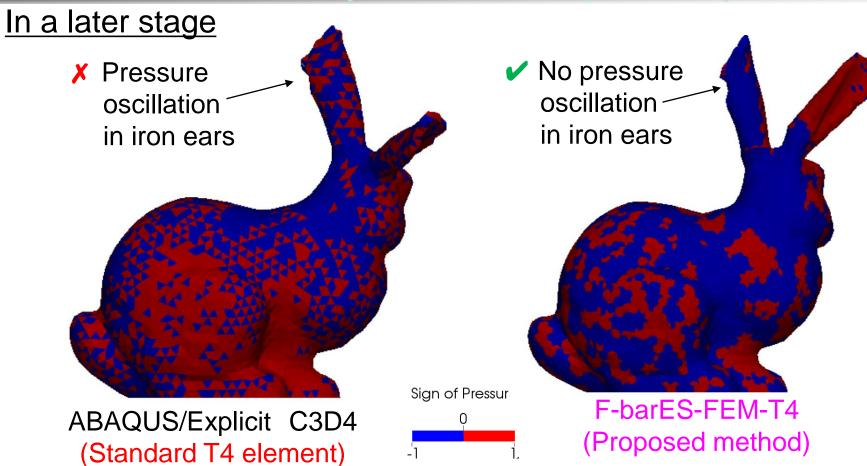
It should be noted that a presence of rubber spoils over all accuracy of the analysis with Standard T4 elements.
