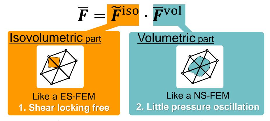
**3. Volumetric locking free** with the aid of F-bar method
